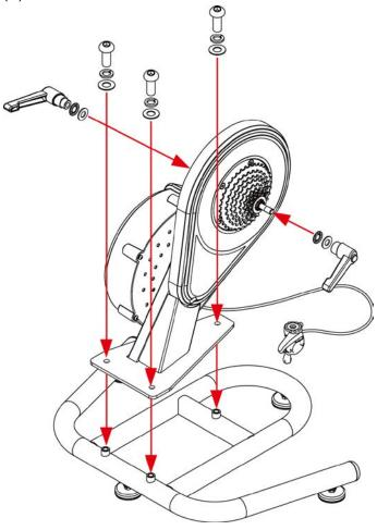
• If the ground is uneven, the leveler may be adjusted until the machine is horizontal. Please make the 4 levelers stay in contact with the ground!
