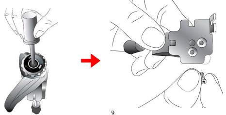
Step2. Turn the fixed piece and align it with the groove; replace the small screw and tighten it. Then turn the resistance lever assembly to the proper position, and tighten the top screw.
