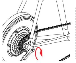
The tightening knob has spring-loaded function, and it may be pulled outward and rotated as needed.
