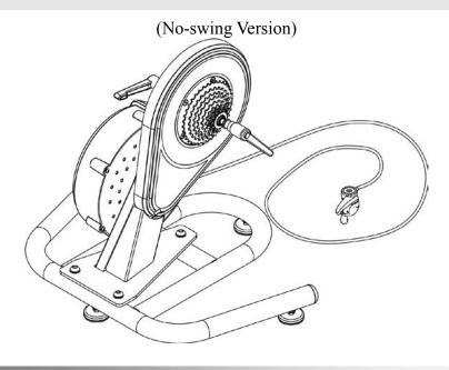
Thank you for purchasing our product. This trainer uses a direct mount of your bicycle's drivetrain to the resistance unit, eliminating tire slippage and wear.
