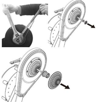
【Step2.】 Use chain whip and cassette lockring tool to remove the lockring.
