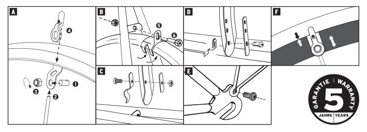
Before mounting the endcap 4, guide the stays through the bridge and eyebolt. The eyebolt should only be tightened slightly. Now set the optimal alignment of the wheel guard to the tire. Mark the appropriate length and cut the stays with a hacksaw.
