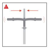
Finally to check the stem is secure, place the front wheel between your legs and twist the handlebars. If there is movement further stem bolt tightening is needed \*\*
