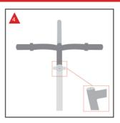
At present the handlebars should be at a **90° angle** to the front wheel and the bolt at the top of the stem in sight.
