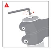
Tighten the headset bolt until pressure is felt using the allen key provided.
