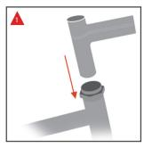
Slot the shaft of the handlebar stem into the hole of the fork's steerer tube.
