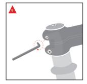
When the headset is tight, check that the handlebars are still 90° to the front wheel and tighten down the stem bolts to secure stem into position.
