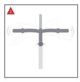
Line up the handlebar \* so that from above, it is at a 90° angle to the front wheel.
