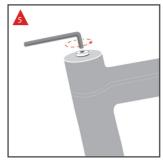
Tighten the bolt with the allen key provided, until resistance is felt. Reattach plug if needed.
